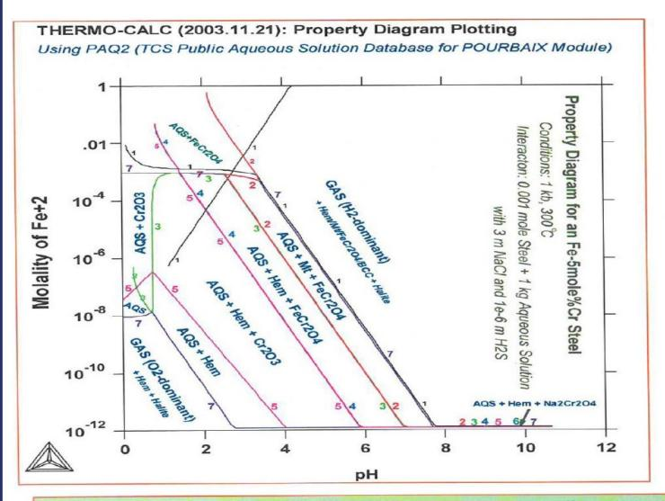
Property Diagrams: Many types of relevant property diagrams, using various X-/Y-axis variables, can be generated from a single POURBAIX-module calculation.
