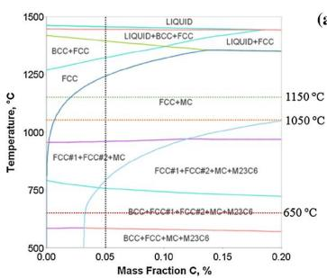
Above: Isopleth section showing that even with variation in carbon, a large FCC+MC carbide region can be found to perform homogenization treatment Right: XRD scan on heat treated build, along with EDS maps of the microstructure.
