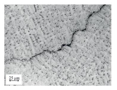
Left: Solidification crack along solidification grain boundary in Nibase alloy weld
