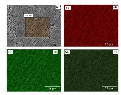
EDS Scans showing segregation of elements across dendrites in 17-4 PH Additive build
