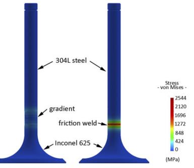
FIG. 5. A finite element model showing elastic mismatch in two dissimilar metal automobile valve stems at 1000 K. The figure on the left shows a valve with a 304L stainless steel stem connected to an Inconel 625 valve via a 2.5 cm long gradient of composition. On the right, the gradient is replaced with a friction weld. The stress at the joint of the friction welded part has an approximately ten times higher stress than the compositionally graded alloy.
