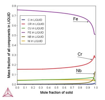
Above: Scheil simulation in Thermo-Calc showing segregation of elements during solidification
