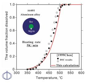
Dissolution of Mg2Si precipitate in Alloy A6401
