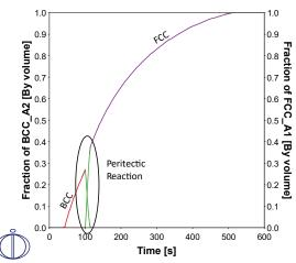
Fraction solid calculated for moving phase boundaries during solidification under full consideration of diffusion in all solid and liquid phases. The peritectic reaction takes about 10 seconds to complete for the chosen cooling rate.
