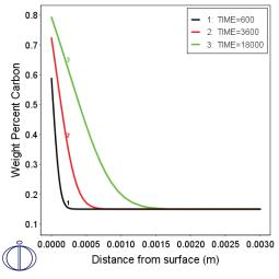
Carbon profiles during carburization of low alloy steel
