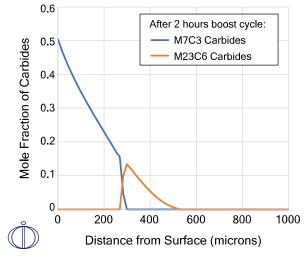
Formation of precipitate carbides of a martensitic stainless steel
