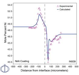
Interdiffusion between a NiAl coating on IN939 at 1050 °C after 96 hours, simulated using the Diffusion Module (DICTRA). The calculation is compared to experimental data from E. Perez, T. Patterson and Y. Sohn, J. Phase Equilibria and Diffusion 27 (2006), pp. 659-64.
