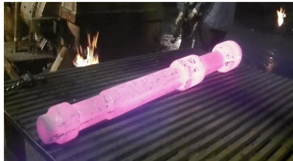
Figure 4. Forged Ferrium M54 Hook Shank
