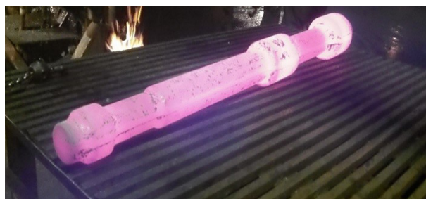
Figure 1a. Completed Ferrium M54 steel T-45 hook shank [NAVAIR Public Release #2014-712 Distribution Statement A-“Approved for public release, distribution is unlimited.”]
