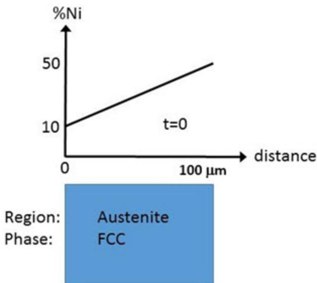
*Schematic view of the initial state of Single Phase Diffusion example. The width of the domain is 100  $\mu\text{m}$  and there is a linear gradient in composition going from 10 to 50 mass-% Ni. There is a single region named Austenite that consists of an fcc phase.*
