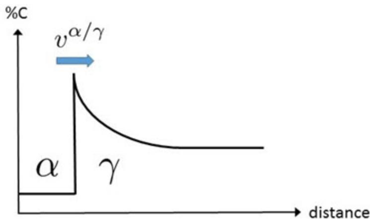
*Schematic view of the carbon profile during the transformation from austenite ( $\gamma$ ) to ferrite ( $\alpha$ ) in the Moving Boundary example.*
