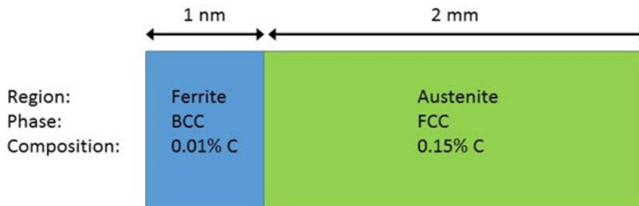
*The set-up of the Moving Boundary example. There are two regions, Ferrite and Austenite, consisting of bcc and fcc, respectively.*
