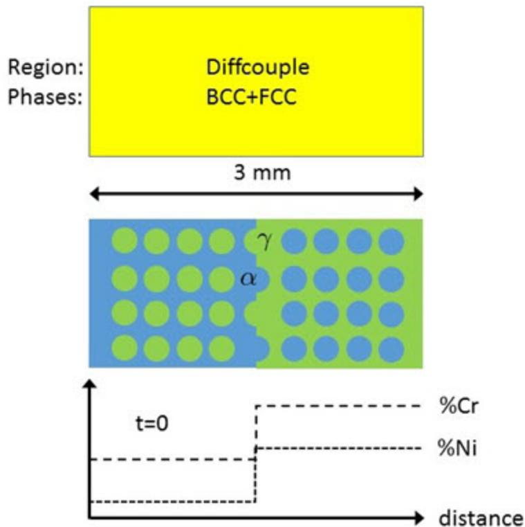
*Schematic view of the initial state of the Multiphase example. Two ternary Fe-Cr-Ni alloys form a diffusion couple. There is a single region (diffcouple) where both the bcc and fcc phases are entered. Both alloys are duplex bcc+fcc, but the majority phase is bcc ( $\alpha$ ) in the left-hand side alloy and fcc ( $\gamma$ ) in the right.*
